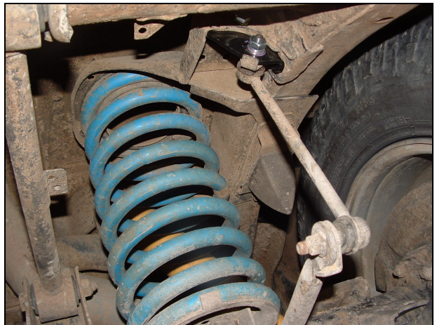
Left hand bracket installed
