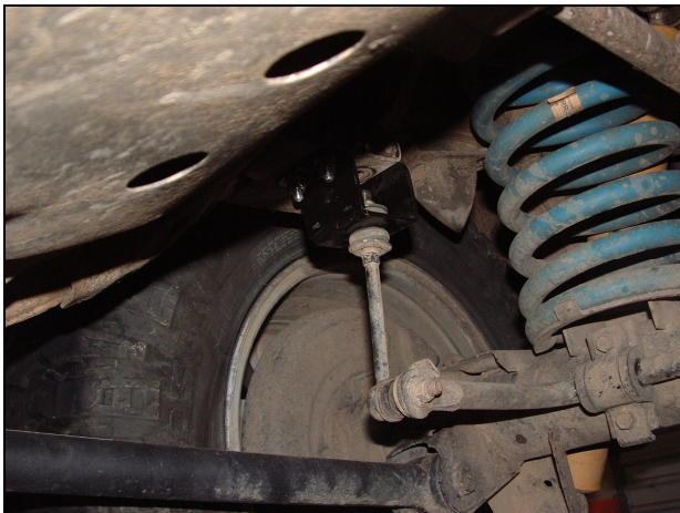
Right hand bracket installed
