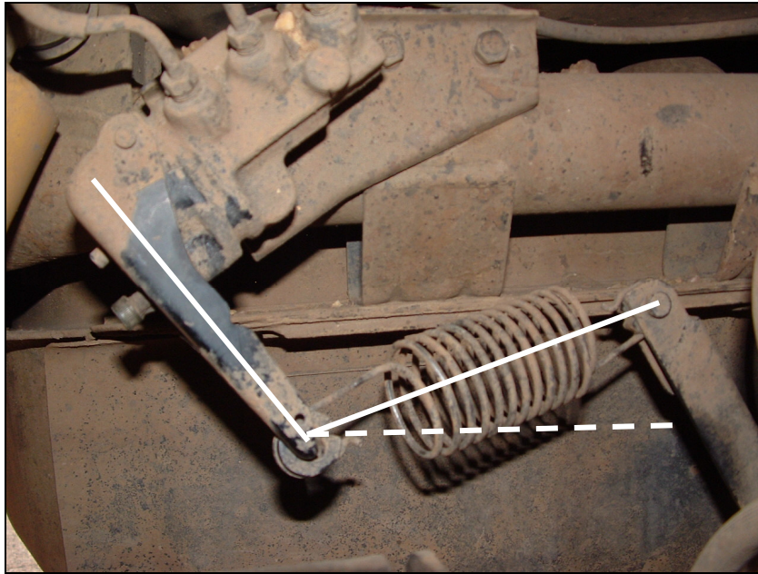
After correction the spring is closer to a 90 degree angle (full line) As opposed to where it was prior to the bracket being fitted (dashed line)
